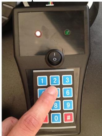
7. After entering the 5-digit code, press the '#' key. The **red** indicator will light steady again.
