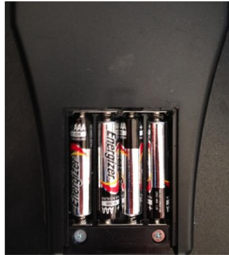
2. Unscrew the keypad from the Sentry Safe unit. There is a small screw at the bottom of the keypad that needs to be unscrewed in order to remove the keypad. Twist the keypad counter-clockwise and pull the keypad unit outward.
