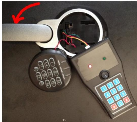
9. Once the safe is opened, you may close back the door and power off the Dumb Safe Opener tool. Disconnect the 4-wire connector from the Dumb Safe Opener tool, and connect it back to the keypad unit. Re-install the keypad unit to the safe and insert back the battery pack. After the beep, enter the 5-digit code used in the safe opener tool. The safe should open now with the new code.
